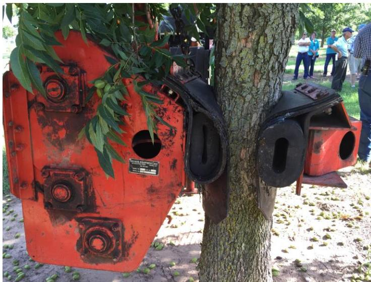
Pecan shaker equipped with donut pads to reduce damage to bark during crop load thinning.
